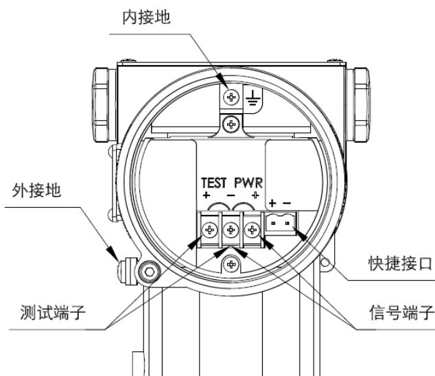
Note: The shortcut interface function is equivalent to the signal terminal
