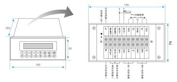
3. Portable mainframe dimensions and wiring diagram
